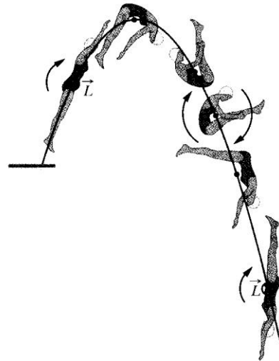
FIG. 11-18 The diver's angular momentum \vec{L} is constant throughout the dive, being represented by the tail \otimes of an arrow that is perpendicular to the plane of the figure. Note also that her center of mass (see the dots) follows a parabolic path.
