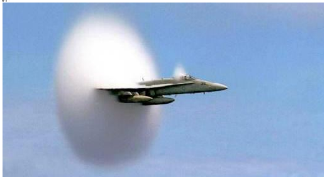
FIG. 17-24 Shock waves produced by the wings of a Navy FA-18 jet. The shock waves are visible because the sudden decrease in air pressure in them caused water molecules in the air to condense, forming a fog. (U.S. Navy photo by Ensign John Gay)
