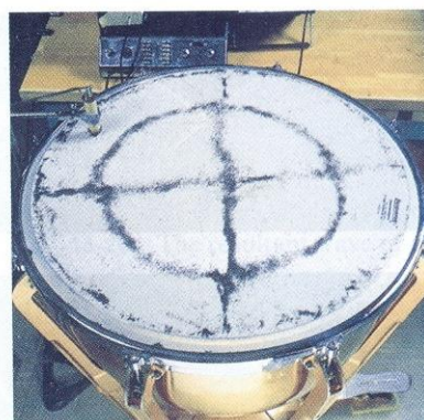
FIG. 16-24 One of many possible standing wave patterns for a kettle-drum head, made visible by dark powder sprinkled on the drumhead. As the head is set into oscillation at a single frequency by a mechanical oscillator at the upper left of the photograph, the powder collects at the nodes, which are circles and straight lines in this two-dimensional example. ( Courtesy Thomas D. Rossing, Northern Illinois University )
