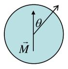
By the way, the B-field inside the sphere is  $\vec{B} = \frac{2}{3} \mu_0 \vec{M}$ , outside the sphere it is the same as due to a pure dipole  $\vec{m} = \frac{4}{3} \pi R^3 \vec{M}$ . (Eq. (3)) <u>ans.</u>
