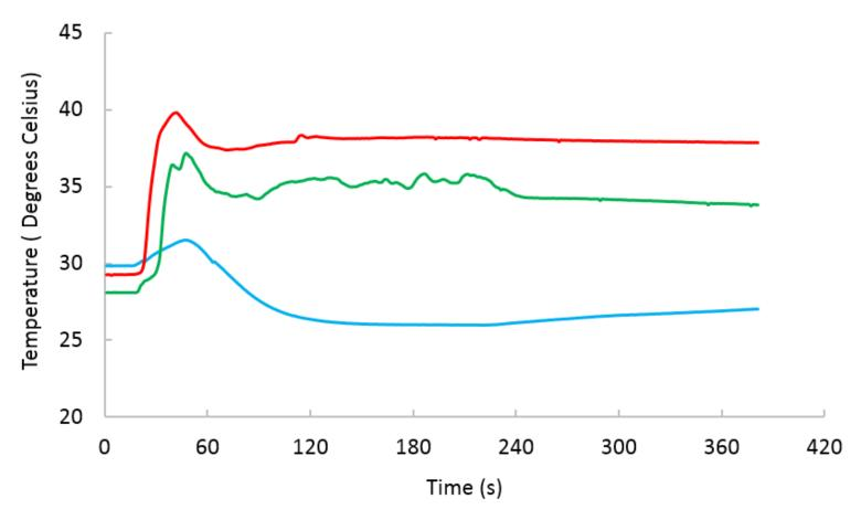
34 litres water used in 381 s; Mass flow rate = 34 kg/381 s = 0.0892 kg/s20 litres LPG =  $0.020 \text{ m}^3$  at calorific value of 26 kWh/m<sup>3</sup>; Energy input =  $26 \times 0.020 \text{ m}^3 = 0.52 \text{ kWh}$ .
