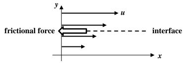
Let  $\tau$  be the average time between successive collisions of a gas molecule with other molecules. Molecule i moves with velocity  $\bar{v}_i$  in random directions, and the average velocity at height y is  $\bar{u}(y)$ .
