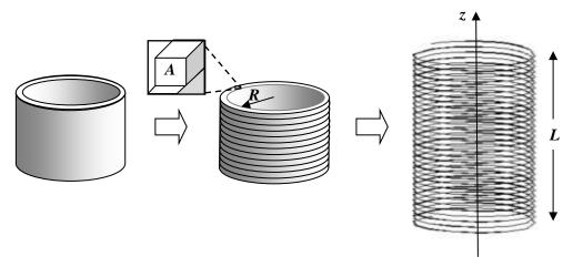
The slinky is a spring first put on sale in 1940's, and soon became a popular toy. As shown in the figure, a slinky can be manufactured from a hollow metal cylinder of radius R by cutting it into a helical thin strip. The helix consists of N turns and has a cross sectional area A. Let  $\rho$  be the density of the metal.
