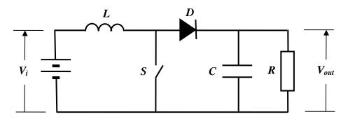
The circuit consists of an input voltage  $V_i$ , an inductor of inductance L, a capacitor of capacitance C, and a load of resistance R. D is a diode whose resistance is effectively zero when the electric potential is higher on the left end, and effectively infinite when the electric potential is lower on the left end.
