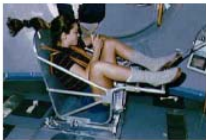
Astronaut Tamara Jernigan measures her inertial mass aboard the Space Shuttle. (NASA)
