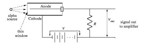
Figure 1 : Schematic diagram of ionization chamber circuit.
