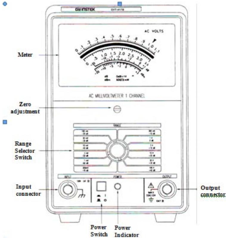
Connect BNC type cable from Amplifier Adaptor to INPUT terminal.
