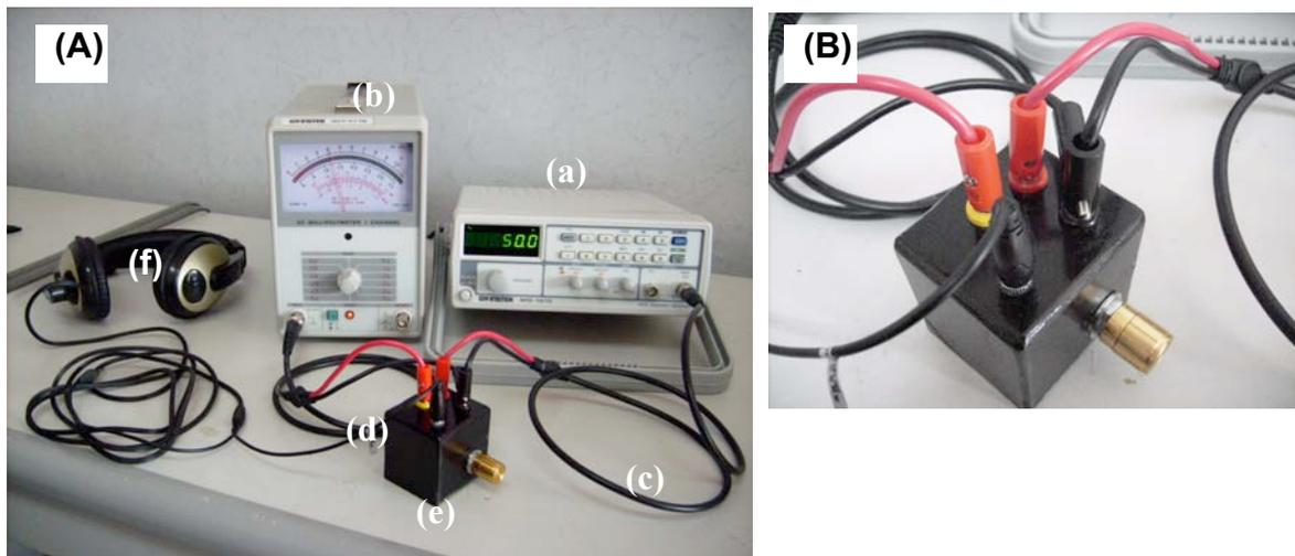
**Figure 4.1 (A).** Connections of the apparatuses. **(B)** Connections of the leads to the rheostat: plug in the red lead from the function generator to the red socket and black lead to the black socket; connect the red lead of AC millivoltmeter to yellow socket and the black lead to the black socket; and plug in headphone lead to the headphone socket.
