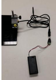
Figure 11: Laser diode mounted inside the laser holder
