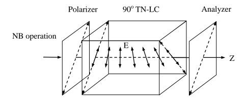
Fig. 9 NB mode operation of a 90° TN cell
