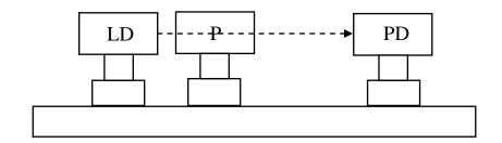
Fig. 6 Alignment of the polarizer (P: polarizer).
