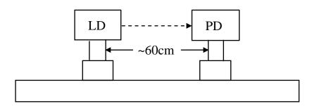
Fig. 4 Optical setup (LD: laser diode; PD: photodetector).
