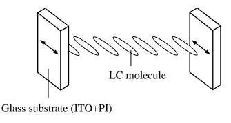
Fig. 10 Homogeneous parallel aligned LC
