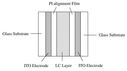
Fig. 7 LC cell structure
