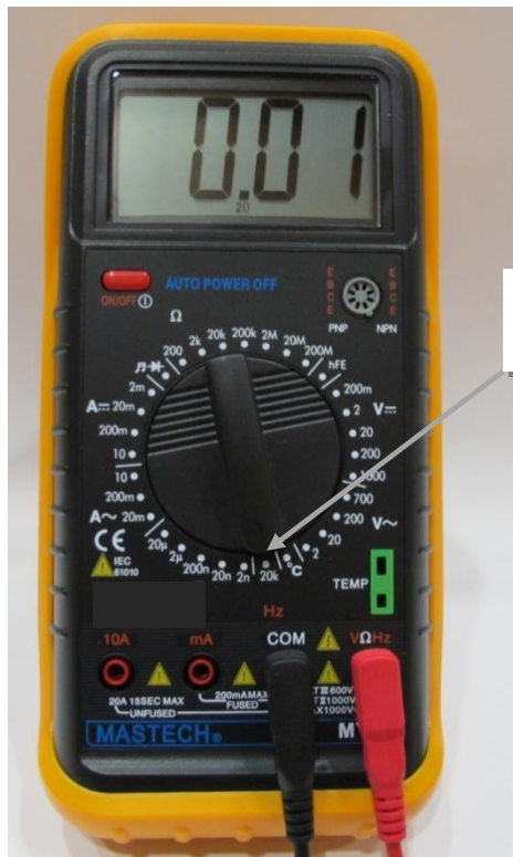
FIGURE 3 Digital multimeter for measuring frequency
