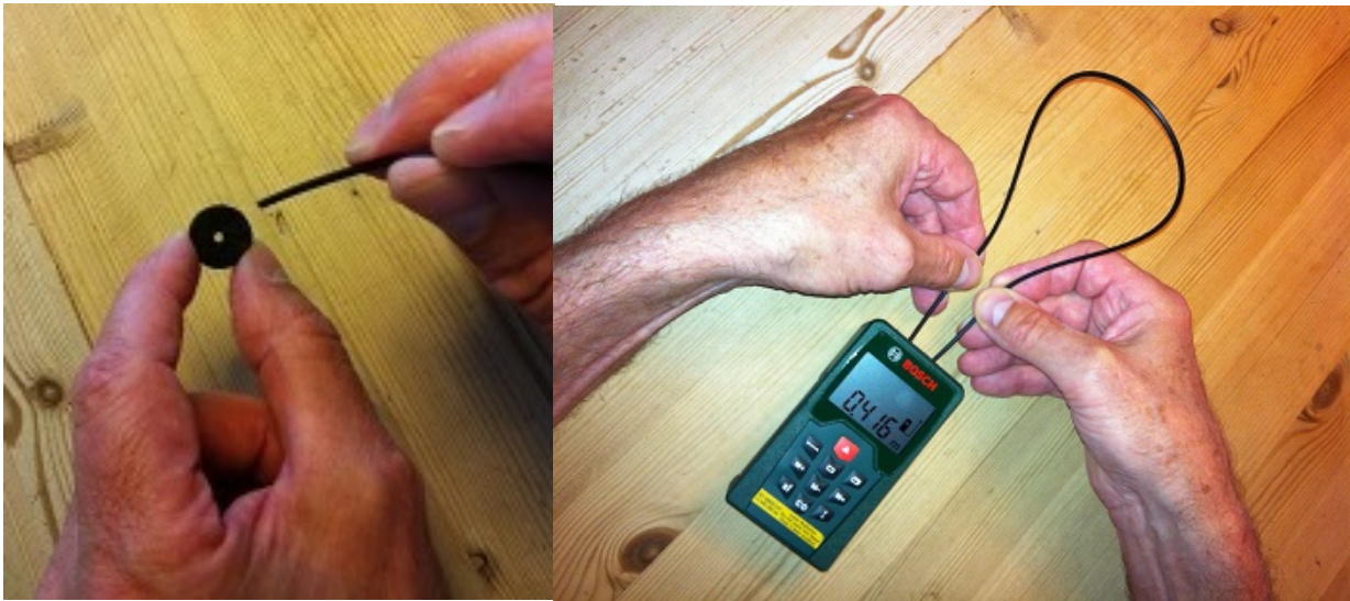
Figure 1.5 (a) Felt pad and fiber optic cable. (b) Attaching the fiber optic cable.
