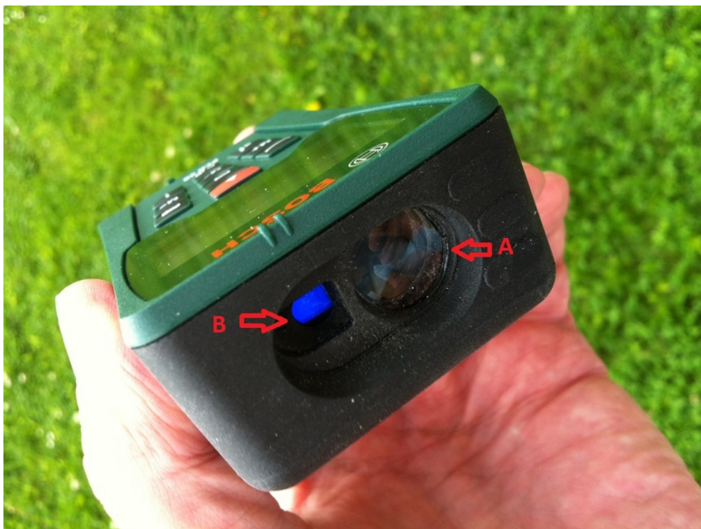
Figure 1.3 The laser distance meter seen from the front end:
